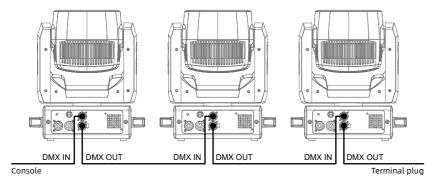
Connect a shielded twisted pair signal cable from the DMX output port of the controller to the DMX input port of the first device, and from the DMX output port of the first device to the DMX input port of the second device, and so on, until all the lamps are connected. Then install a terminal plug on the last 3 or 5 pin socket of each connected lamp output. (Weld a 4/1W, 120  $\Omega$  resistor between the 2 and 3 pins of a 3 or 5 core pin XLR plug).
