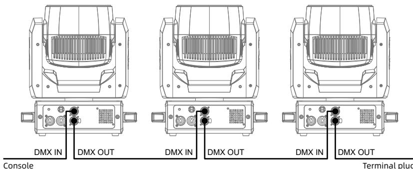
Connect a shielded twisted pair signal cable from the DMX output port of the controller to the DMX input port of the first device, and from the DMX output port of the first device to the DMX input port of the second device, and so on, until all the lamps are connected. Then install a terminal plug on the last 3 or 5 pin socket of each connected lamp output. (Weld a 4/1W, 120 Ω resistor between the 2 and 3 pins of a 3 or 5 core pin XLR plug).
