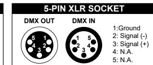
The lighting fixtures are equipped with standard DMX XLR and RJ-45 input and output sockets. Please use DMX512 shielded twisted pair signal cables or Category 5 or above network twisted pair cables for connection. The typical connection distance for DMX signal lines is 150 meters. When transmitting signals over long distances, a DMX512 signal amplifier must be added.
