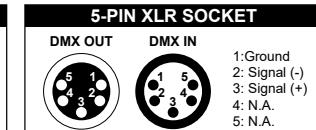
The lighting fixtures are equipped with standard DMX XLR input and output sockets. Please use DMX512 shielded twisted pair signal cables or Category 3/5 or above network twisted pair cables for connection. The typical connection distance for DMX signal lines is 150 meters. When transmitting signals over long distances, a DMX512 signal amplifier must be added.
