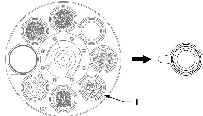
d). Use tweezers or other small grippers to remove the snap spring at point **J** (If the pattern piece is coated with glass glue for fixation, please use a professional cleaning agent to remove the glass glue before removing the snap spring to avoid damaging the gobo);
