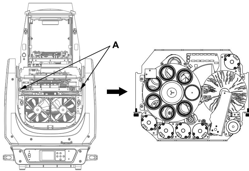
b). As shown in **B**, gently lift the driven wheel from the edge upwards from the front of the pattern plate and slowly pull it out to remove a single pattern seat;
