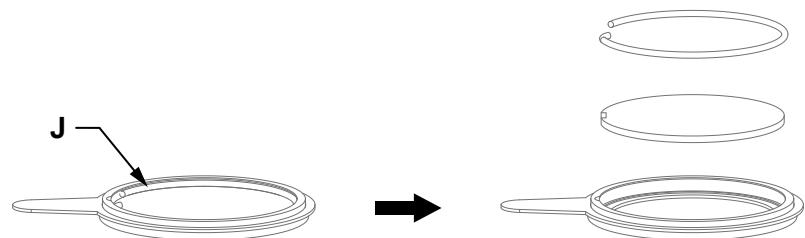
e). When assembling the gobo, avoid touching it directly with your hands. As shown in **K**, align the notch of the gobo with the recess of the driven wheel component (the coating surface of the gobo should face the light source);
