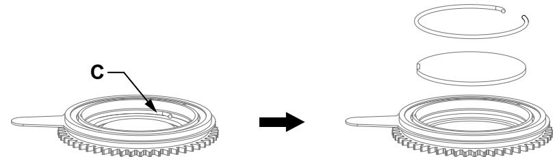
d). When assembling the gobo, avoid touching it directly with your hands. As shown in D, align the notch of the gobo with the recess of the driven wheel component (the coating surface of the gobo should face the light source);
