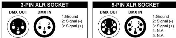
The lighting fixtures are equipped with standard DMX XLR input and output sockets. Please use DMX512 shielded twisted pair signal cables or Category 3/5 or above network twisted pair cables for connection. The typical connection distance for DMX signal lines is 150 meters. When transmitting signals over long distances, a DMX512 signal amplifier must be added.
