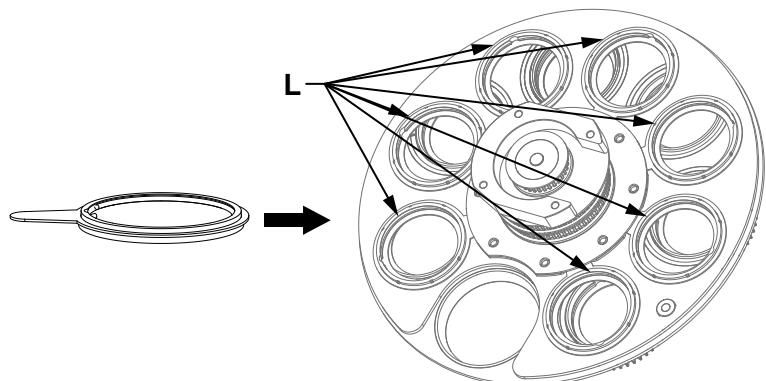
g). After installation, simply reinstall the gobo wheel component onto the light fixture.
