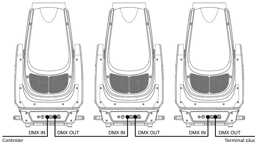
Connect a shielded twisted pair signal cable from the DMX output port of the controller to the DMX input port of the first device, and from the DMX output port of the first device to the DMX input port of the second device, and so on, until all the lamps are connected. Then install a terminal plug on the last 3 pin socket of each connected lamp output. (Weld a 4/1W, 120 Ω resistor between the 2 and 3 pins of a 3 or 5 core pin XLR plug).
