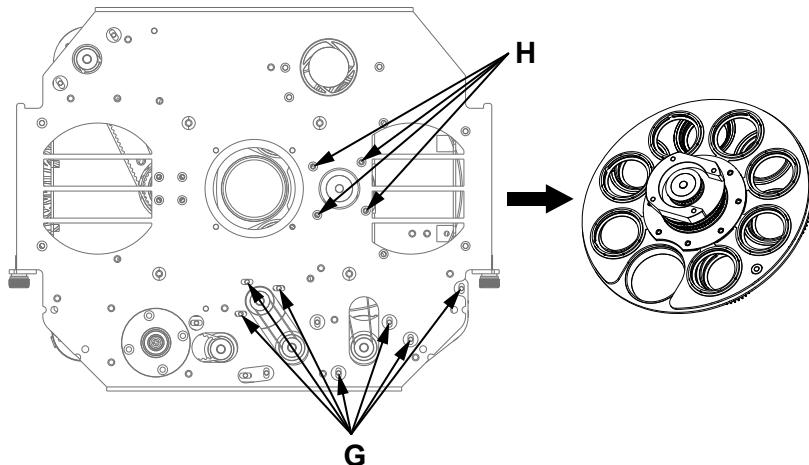
c). As shown in **I**, gently lift the gobo holder from the edge of the gobo wheel 2 and slowly pull it out to remove a single gobo holder;
