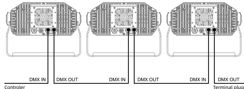
Connect a shielded twisted pair signal cable from the DMX output port of the controller to the DMX input port of the first device, and from the DMX output port of the first device to the DMX input port of the second device, and so on, until all the lamps are connected. Then install a terminal plug on the last 3 pin socket of each connected lamp output. (Weld a 4/1W, 120 Ω resistor between the 2 and 3 pins of a 3 or 5 core pin XLR plug).
