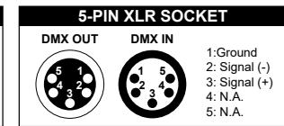
The lighting fixtures are equipped with standard DMX XLR input and output sockets. Please use DMX512 shielded twisted pair signal cables or Category 3/5 or above network twisted pair cables for connection. The typical connection distance for DMX signal lines is 150 meters. When transmitting signals over long distances, a DMX512 signal amplifier must be added.
