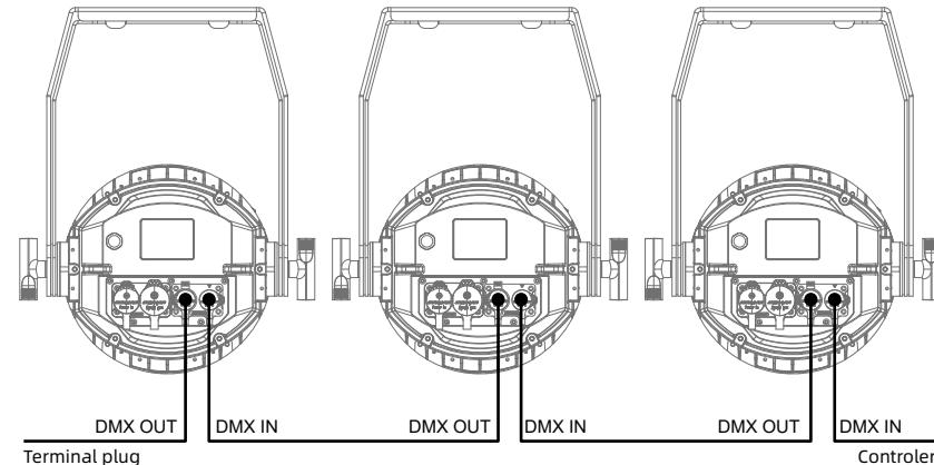
Connect a shielded twisted pair signal cable from the DMX output port of the controller to the DMX input port of the first device, and from the DMX output port of the first device to the DMX input port of the second device, and so on, until all the lamps are connected. Then install a terminal plug on the last 3 pin socket of each connected lamp output. (Weld a 4/1W, 120 Ω resistor between the 2 and 3 pins of a 3 or 5 core pin XLR plug).
