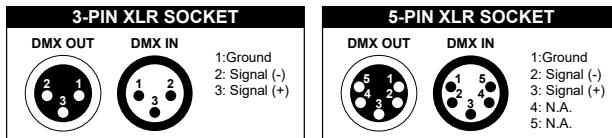
The lighting fixtures are equipped with standard DMX XLR input and output sockets. Please use DMX512 shielded twisted pair signal cables or Category 5 or above network twisted pair cables for connection. The typical connection distance for DMX signal lines is 150 meters. When transmitting signals over long distances, a DMX512 signal amplifier must be added.
