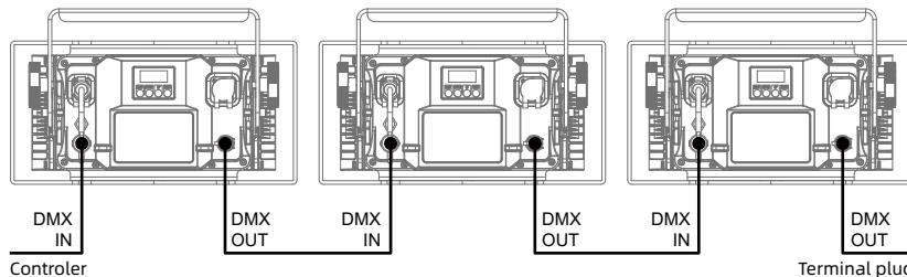
Connect a shielded twisted pair signal cable from the DMX output port of the controller to the DMX input port of the first device, and from the DMX output port of the first device to the DMX input port of the second device, and so on, until all the lamps are connected. Then install a terminal plug on the last 3 pin socket of each connected lamp output. (Weld a 4/1W, 120 Ω resistor between the 2 and 3 pins of a 3 or 5 core pin XLR plug).
