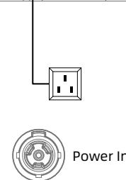
**Attention:** When connecting the power supply, the ground wire (yellow/green dual color wire) must be safely grounded and comply with all relevant electrical installation standards.
