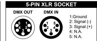
The lighting fixtures are equipped with standard DMX XLR input and output sockets. Please use DMX512 shielded twisted pair signal cables or Category 3/5 or above network twisted pair cables for connection. The typical connection distance for DMX signal lines is 150 meters. When transmitting signals over long distances, a DMX512 signal amplifier must be added.
